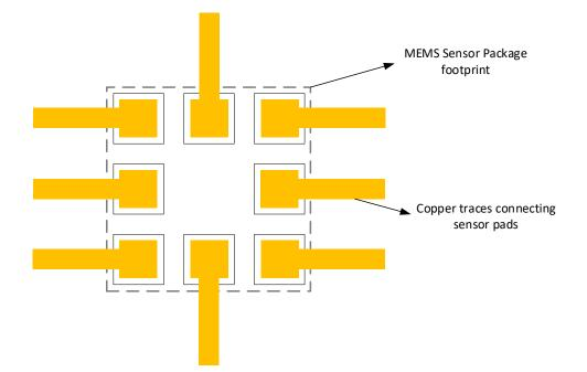
Figure 7: Symmetrical trace and sensor pad connections
