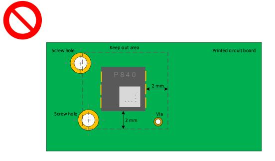
Figure 4: Components inside sensor keep out area
