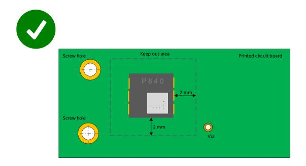
Figure 5: Components outside sensor keep out area
