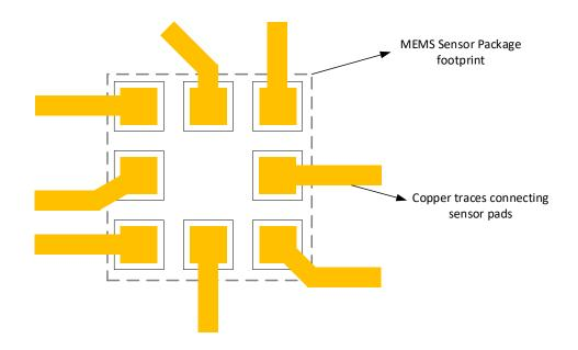
Figure 6: Asymmetrical trace and sensor pad connections
